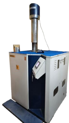
Figure 2: A typical Gamma-cell Irradiator (Uses ^{60}\text{Co} as source)
